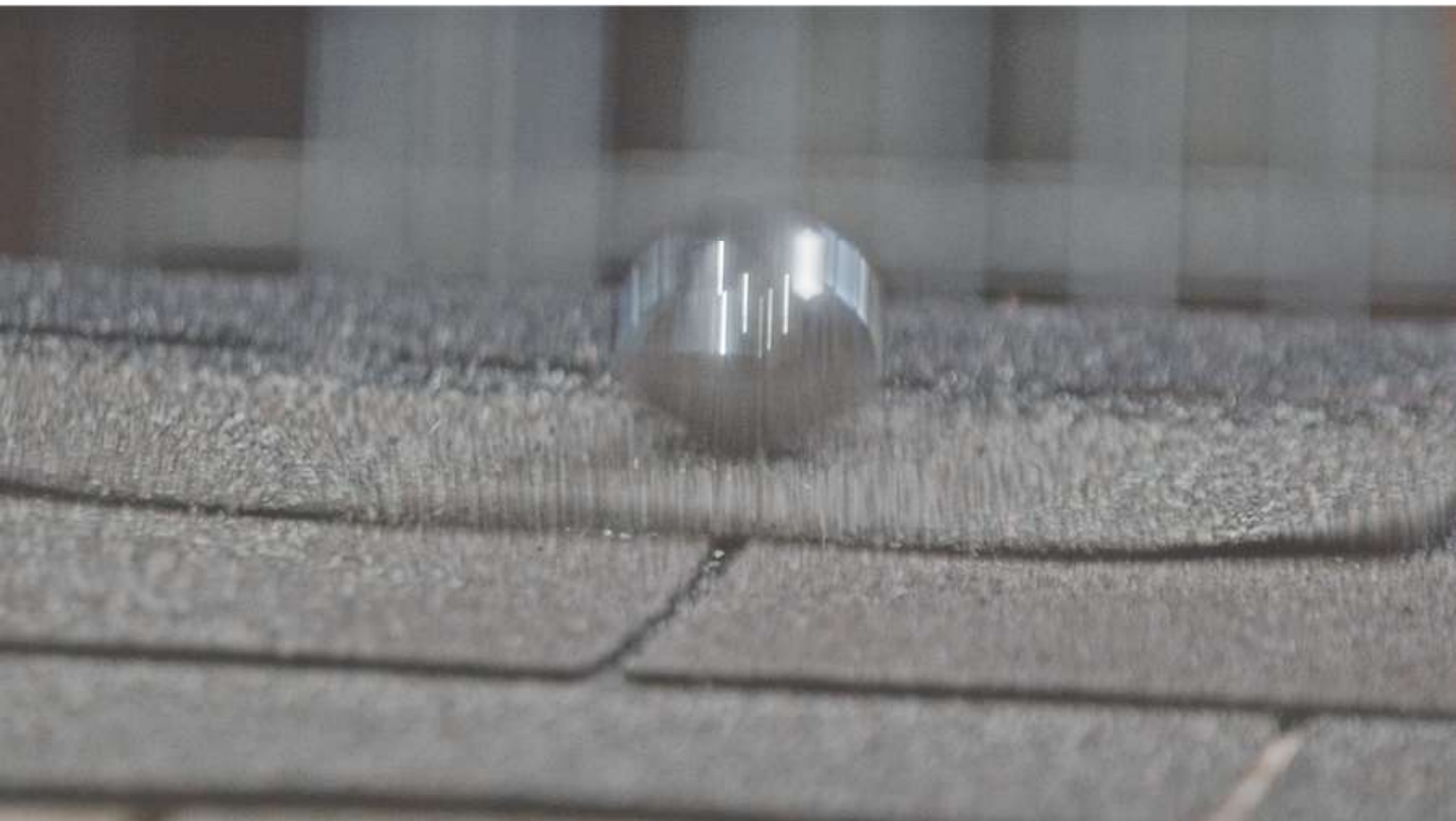
2" Steel Ball Drop from 20' High - Granules Stay Bonded to Shingle
